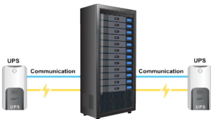
Some systems have multiple power supplies and cords. You typically find this on high-end servers that allow hot-swap and other fun features. In this case, you run multiple drivers (one per UPS), a single `upsd`, and a single `upsmmon` (as a primary for both UPS 1 and UPS 2)
